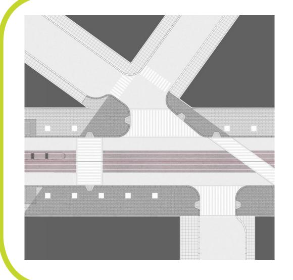
Market Street has uniquely oblique intersections. The sidewalk paving design will highlight this characteristic through paving color and texture.
